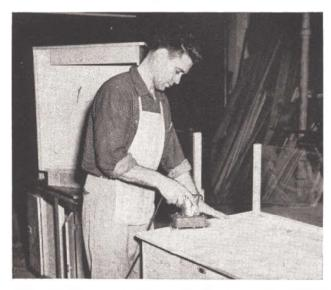
Most attachments fit all standard makes and models. Orbit sander adapts to any ¼-inch electric drill.
