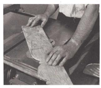
Scroll saw here fits tilting arbor circular saw, cuts angle curves; also saws, files, sands metal, plastic.
