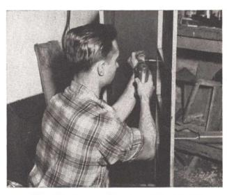
Specialized shop operations are made easy with lowpriced power-tool attachments like this angle head.
